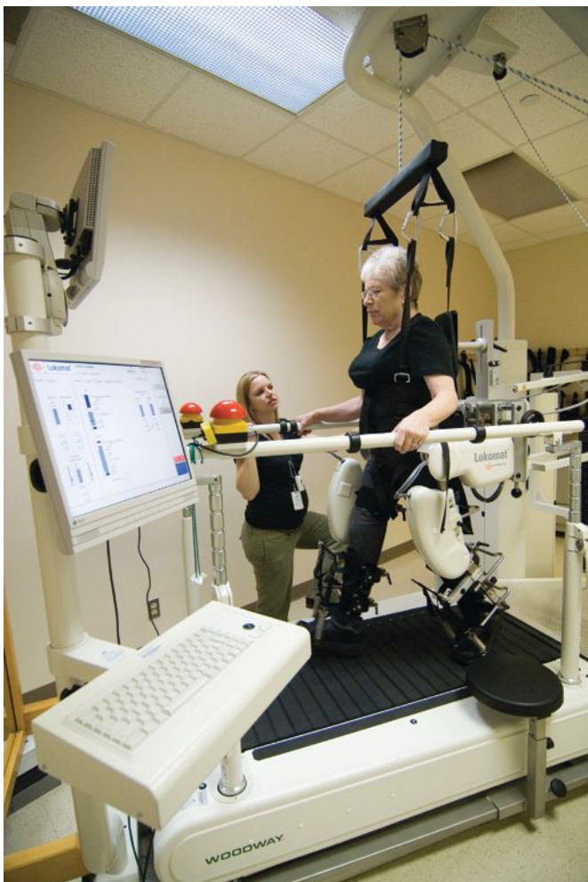
A robot-assisted treadmill supports the patient in an upright position while moving the legs through a normal walking pattern.
