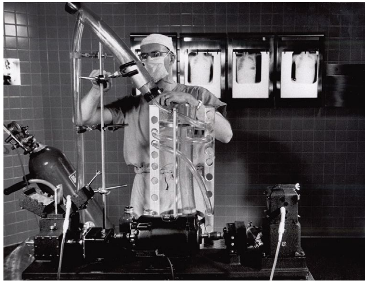
Richard DeWall operating his invention, the DeWall Bubble Oxygenator, for use during open heart surgery circa 1956.
