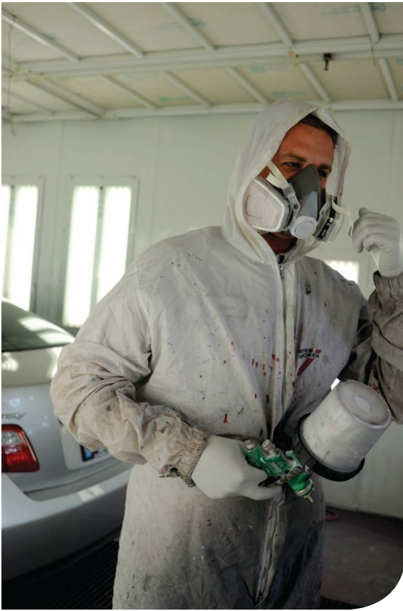
One way to protect the health of collision repair workers is to make sure they wear properly fitted respirators when they are using potentially harmful chemicals.
